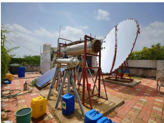
Pilot plant model using solar energy – Sea water into potable water
