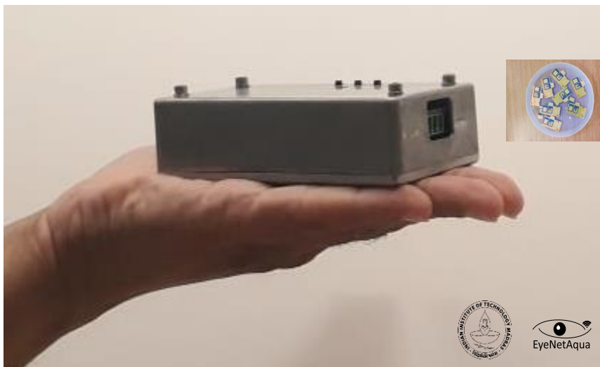
A handheld device for the testing of arsenic using “drop-and-sense” test strips (inset)
