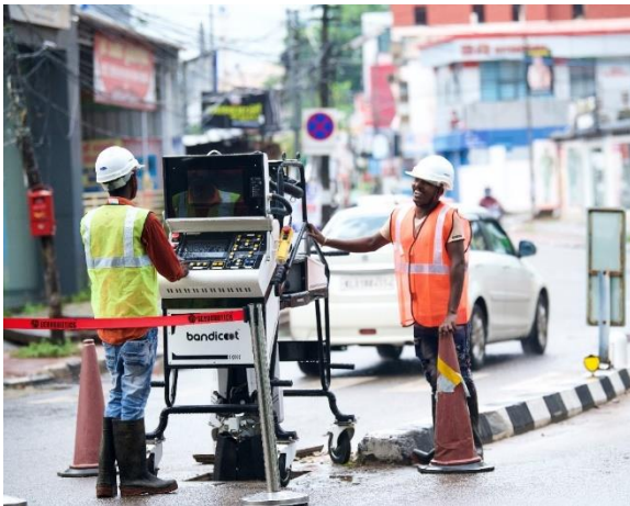
Bandicoot robots for cleaning sewers
