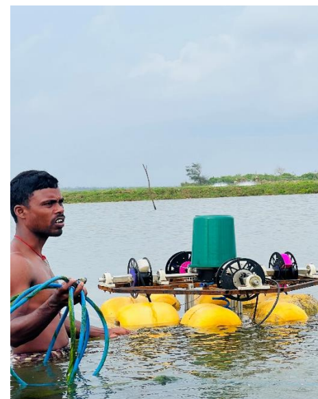
Diffused Flapping Sediment Aeration Device
